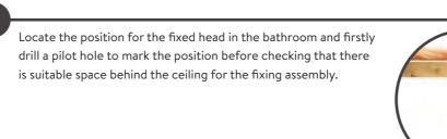
The minimum height required behind the ceiling is 50mm and the space must allow for an 80mm wide, 50mm deep noggin to be used to support the assembly.
