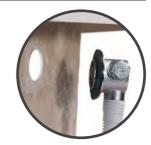
insuring the rubber washer is correctly aligned, pass the overflow filler outlet through the bath and secure to the body assembly.
