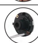
Place the 'O' ring on the recess of the spigot section on the mounting plate, offer the wall outlet onto the mounting plate in the 5 o'clock position and rotate clockwise until a stop is reached.
